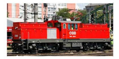
Battery energie storage (LiFePo4) with supercaps for shunting operations without catenary and charging during catenary operation
