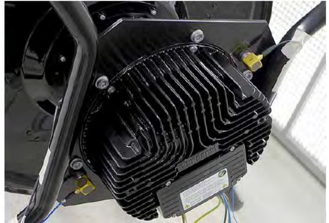
Triaxial Vibrationssensoren auf Ventilator, EBM – Pabst , 2018 in VHK and Viegand Maagøe, ICT Impact study, July 2020, p. 177
