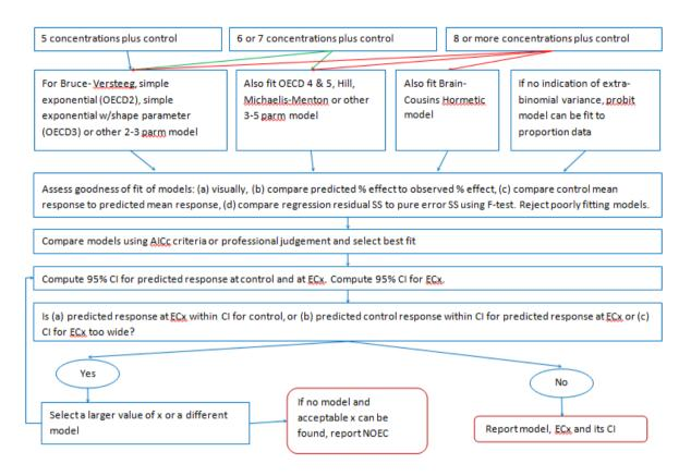
**Figure 4:** Flow chart for EC<sub>x</sub> Estimation of Replicate Mean Length, Weight, or Proportion of Egg Hatch or Larval Mortality, see text for more details
