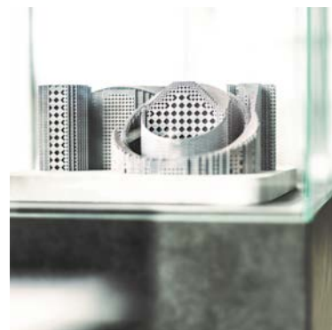
Unique metal PBF support structures
