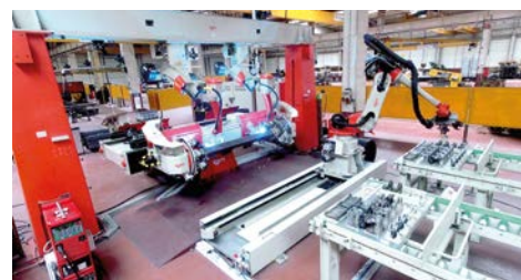
Cooperating robots in welding cell for truck axles
