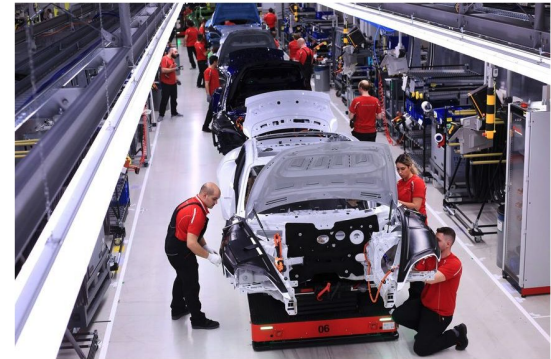
Employees work on the body shells of all-electric Porsche AG Taycan luxury automobiles on the production line inside the company's factory in Stuttgart, Germany, in 2020.
