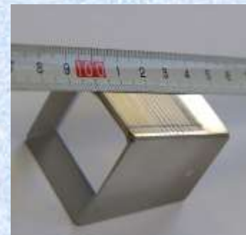
Elements (light-sound waveguides) of paratellurite for all types of acoustooptic devices
