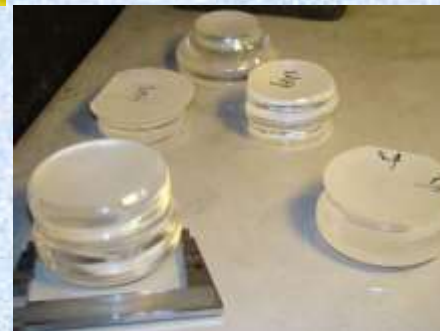
Technology of paratellurite processing (orientation → cutting → grinding → polishing)
