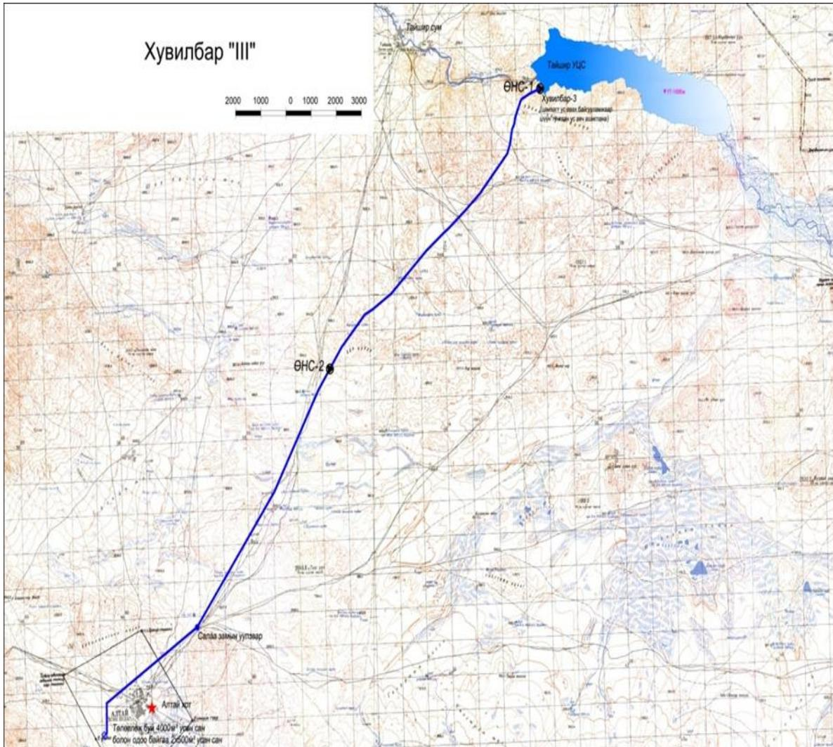
**Figure 1. Selected ductile iron transmission pipeline alignment**
