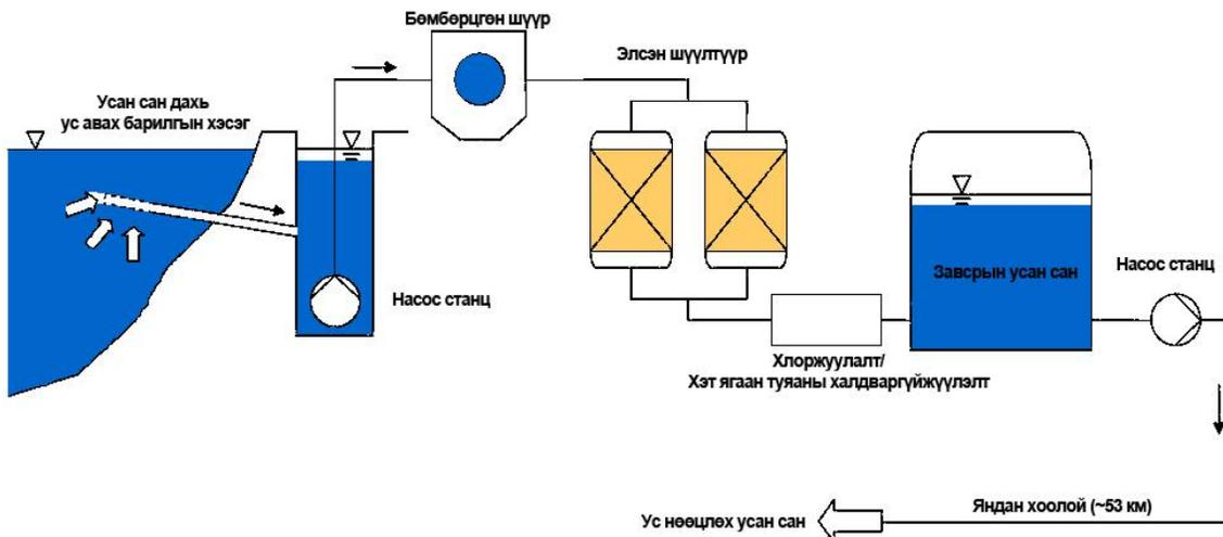
**Figure 4. Simplified diagram of water treatment facility**
