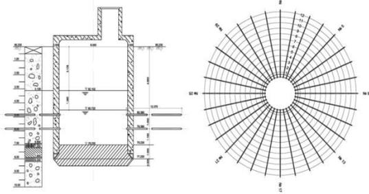
**Figure 2. Underground horizontal radial water intake facility design**
