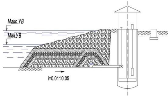
**Figure 3. Underground horizontal water intake facility design**
