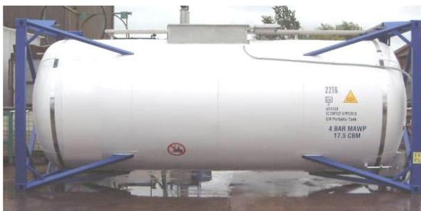
Figure 3.38 – Beam tank no top rail
