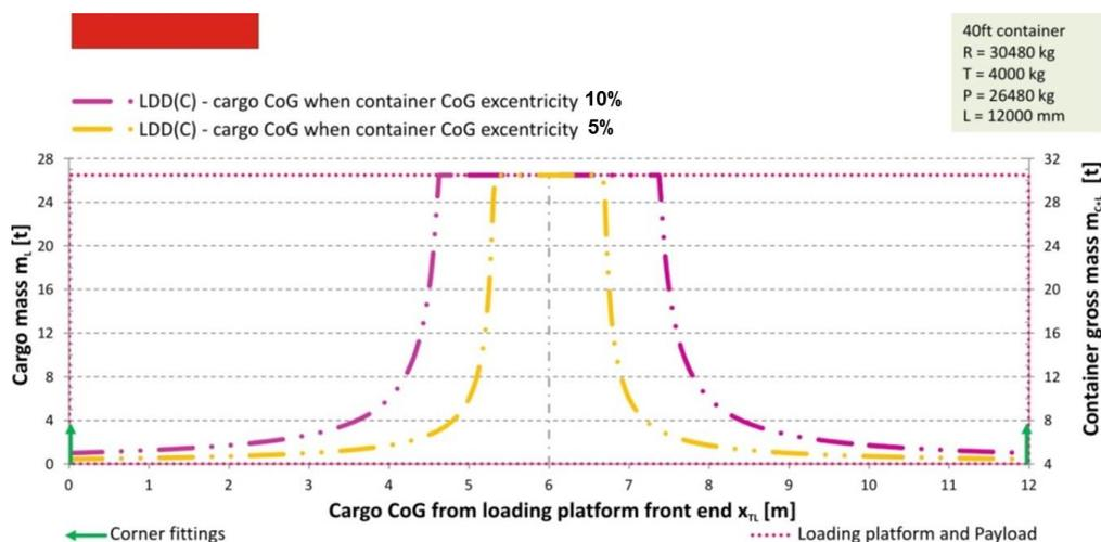
Figure 6.1 – Load distribution diagram for 40-foot container
