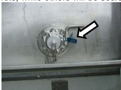
Figure 9.16 Top valve seal
