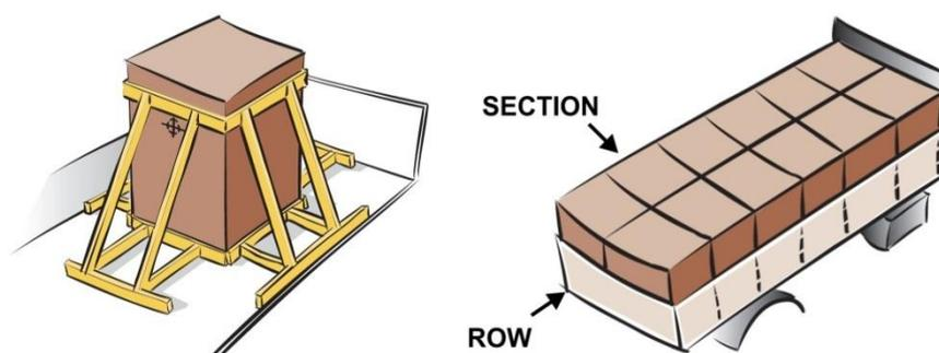
1.1.3 The sum of void spaces in any horizontal direction should not exceed 15 cm. However, between dense rigid cargo items, such as steel, concrete or stone, the void spaces should be further minimized, as far as possible.
