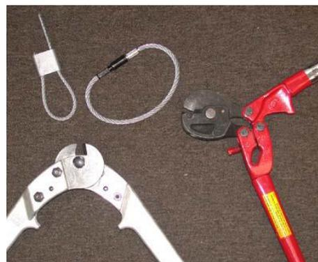
Figure 9.27 High-security Cable seals
