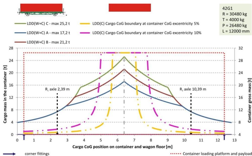
Figure 6.6 – Load distribution diagram of 40-foot container loaded onto a 2 axle wagon
