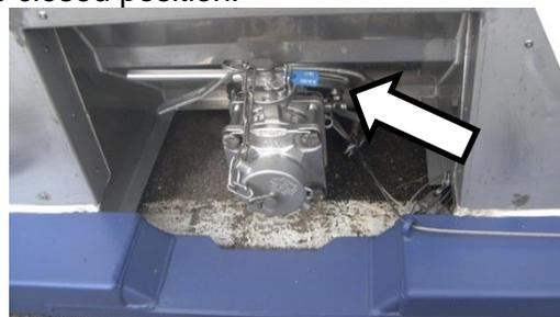
Figure 9.17 Discharge valve seal
