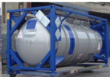
Figure 3.39 – Beam tank with top rail
