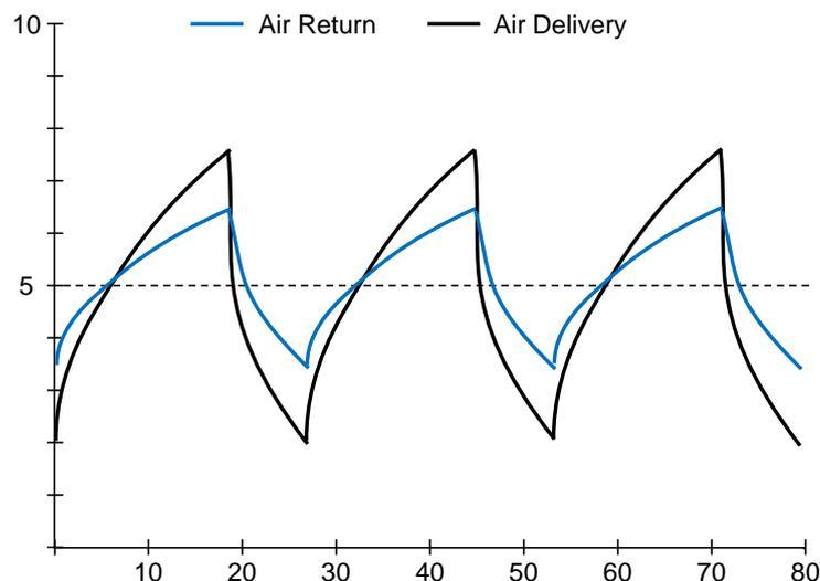
Figure 8.14 Variations of air temperature under thermostatic control
