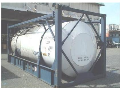
Figure 3.36 – 20,000 l frame tank
