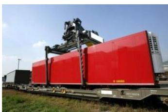
Figure 3.87 – Trailer loading using grapple arms
