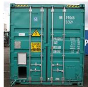
Figure 3.45 – Cat flap type hatch in rear doors
