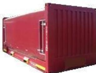
**Figure 3.56 – Covered steel coil carrier**
