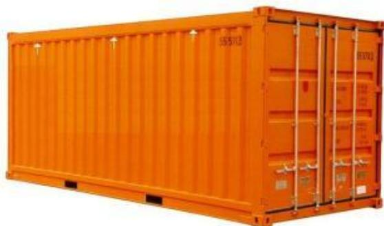
**Figure 3.17 – 20-foot passive ventilated container**
