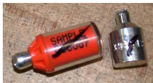
Figure 9.32 Cut bolt seals – head
