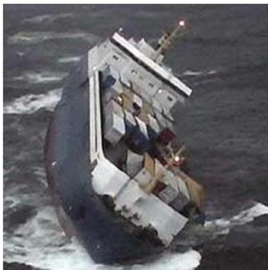
**Figure 1.5 – Heavily listing ship after cargo has shifted**
