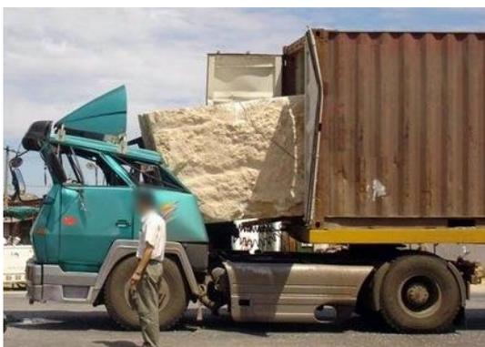
Figure 1.1 – Lack of longitudinal securing
