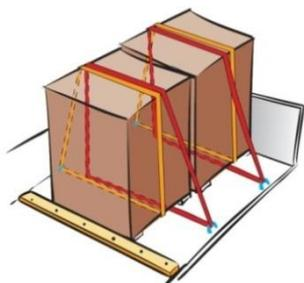
The quick lashing guide shows that a pair of half-loop **web lashings** with MSL 2,000 daN prevents 4.3 tonnes of cargo from sliding sideways in Sea Area C, when the friction factor is 0.3.
