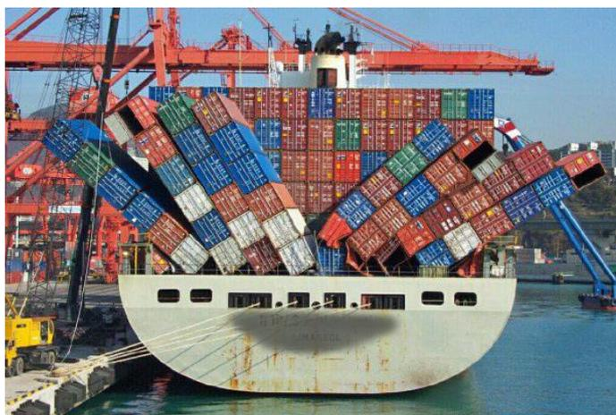
Figure 1.16 – Stack failure
