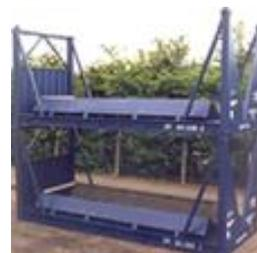
**Figure 3.57 – Open steel coil carrier**
