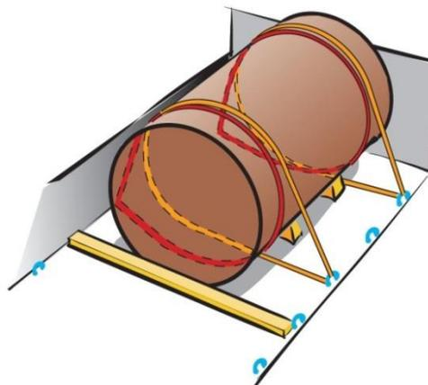
For tipping half the Maximum Securing Load (MSL) value should be used for design purposes.
