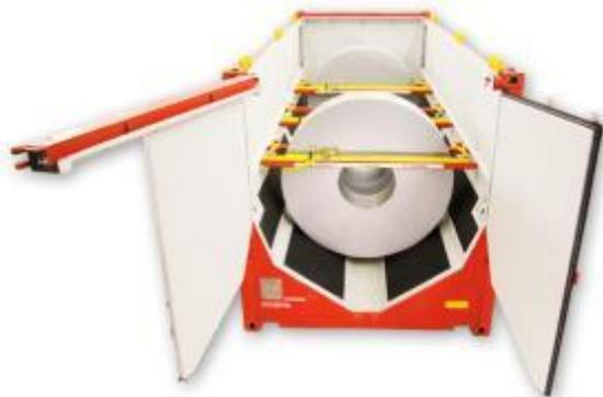
Figure 3.24 – 20-foot coil carrier
