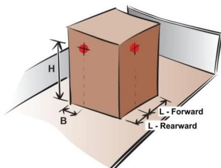
The dimensions **H**, **B** and **L** as indicated to the left should be used in the tables for tipping for cargo units with centres of gravity away from their geometrical centres.
