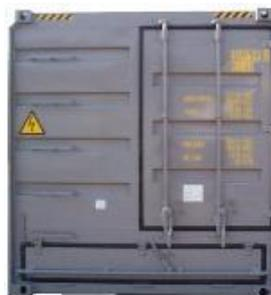
Figure 3.44 – Letterbox type hatch in fixed rear end
