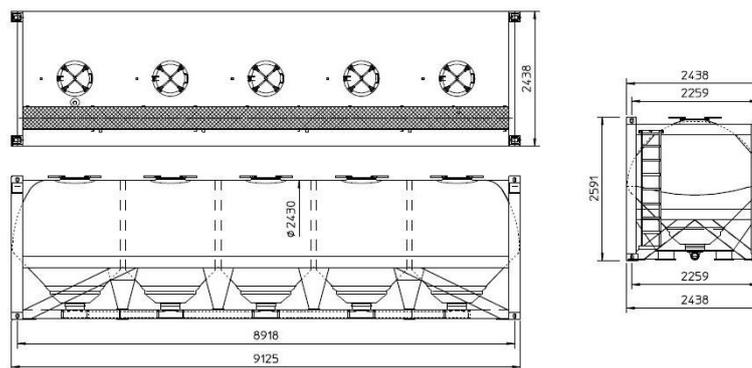
Figure 3.46 – 30-foot hopper type dry bulk container
