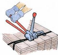
The tables are valid for **steel strapping (32 × 0.8 mm)** with an MSL of 17 kN or 1,700 daN – (1,700 kg = 1.7 tonnes) and a pre-tension of minimum 2.4 kN or 240 daN – (240 kg).
