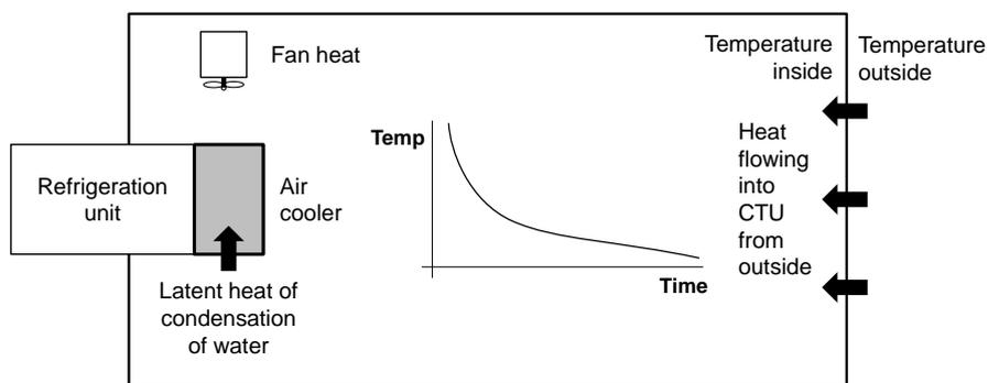
Figure 8.11 Heat load of a refrigerated CTU
