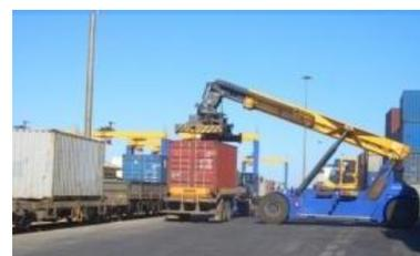
Figure 3.88 – Container loading using reach stacker
