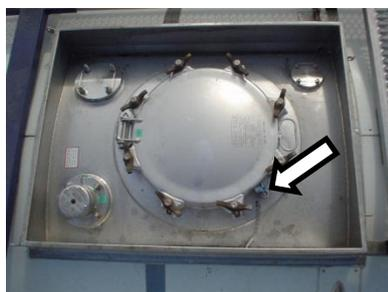
Figure 9.14 Manway hatch seal
