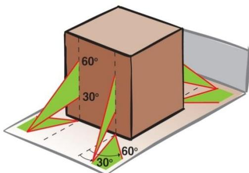
The tables are valid for an angle of 30° to 60° between the lashing and the platform bed.
