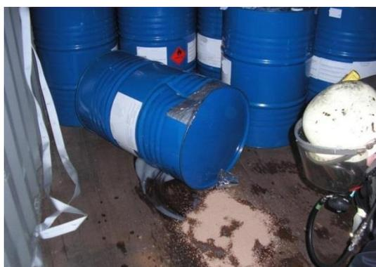
**Figure 1.8 – Spilled liquid dangerous goods**
