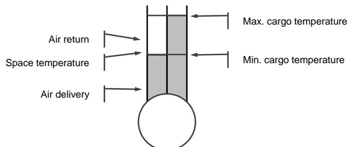
Figure 8.1 Relationship of cargo and air temperature
