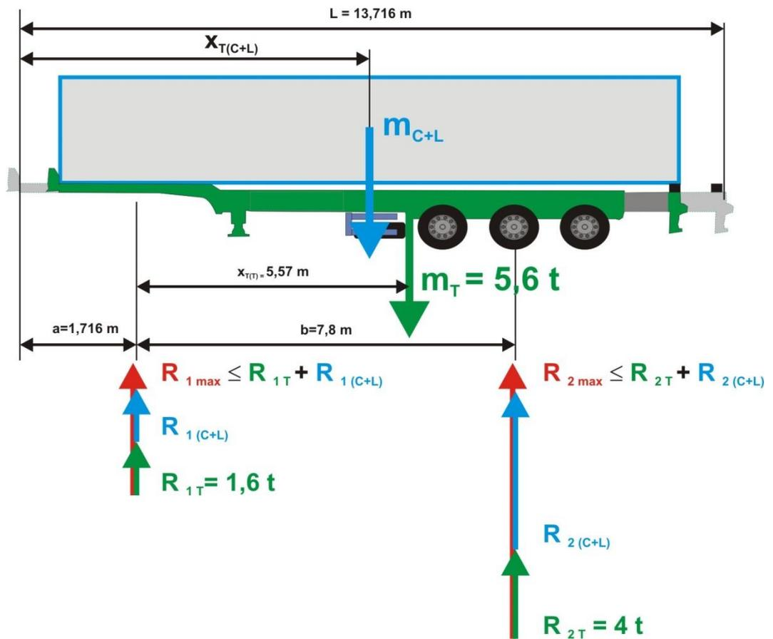
Figure 6.4 – Typical three axle extendable 45-foot container trailer
