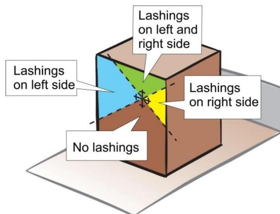
When the lashings are fixed above the centre of gravity, the unit may also have to be blocked at the bottom to prevent sliding.
