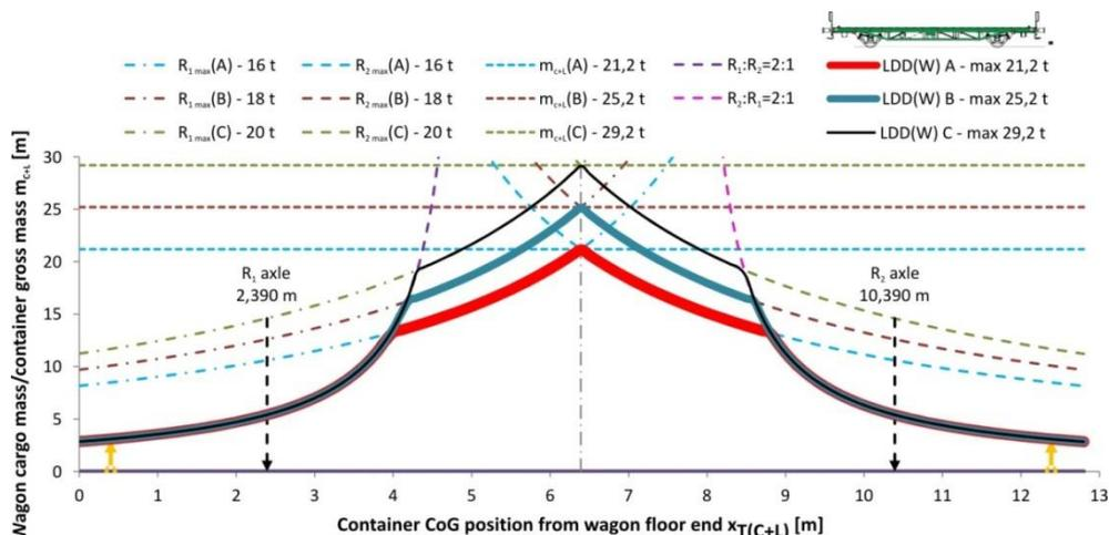
Figure 6.3 Load distribution diagrams (LDD) for container wagon for different route categories
