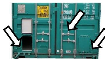
Figure 9.12 Dry bulk discharge hatch (rear)
