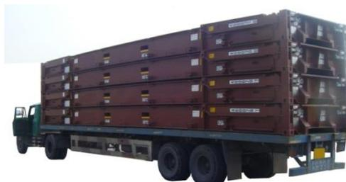
**Figure 3.52 – Stack of 40-foot folding end flatracks**
