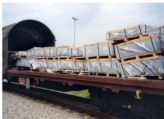
**Figure 1.7 – Loose packages on rail wagon**
