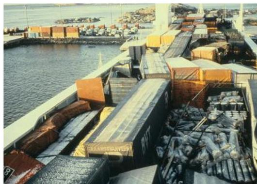
Figure 1.4 – Shifted cargo on a ro-ro deck
