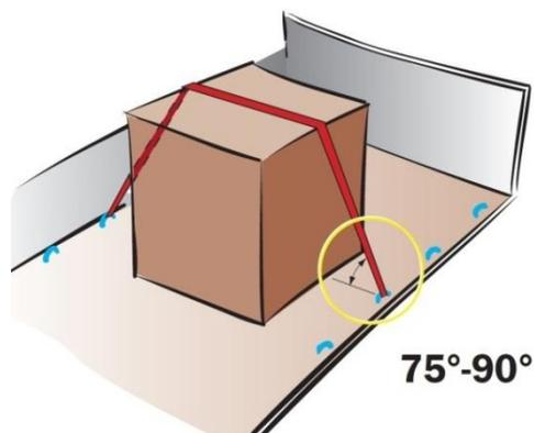
When using the tables for top-over lashing the angle between the lashing and the platform bed is of great importance. The tables are valid for an angle between 75° to 90°. If the angle is between 30° to 75° twice the number of lashings are needed (alternatively the table values are halved). If the angle is less than 30°, another cargo securing method should be used.
