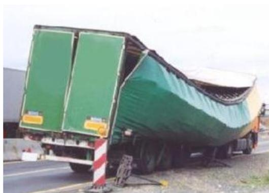
Figure 1.2 – Inadequate side wall strength
