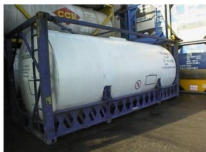
Figure 3.37 – 25,000 l frame tank
