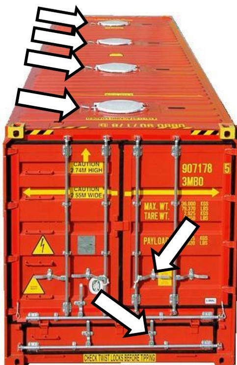
Figure 9.10 Dry bulk sealing points
